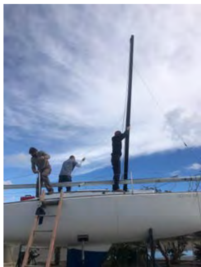
CIYC J24 Teamwork! Dan Maxwell (right) is holding the gin pole while Gareth Jones (left) and Mike Geer (center) sort out the standing rigging and prepare to stand TINY DANCER's mast.
