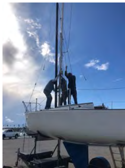
And with the leverage of the gin pole, the halyards, and the crew ..it's up!
